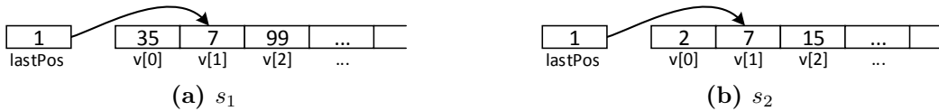
Figure 2.1: Two shared states satisfying the same base condition \Phi_3 : lastPos = 1 \wedge v[1] = 7 .
